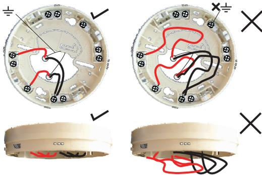
Wires should be of minimal excess length and be pushed back flat inside the base.
