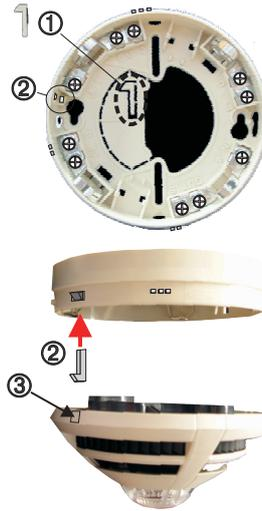
Remove the locking peg from cutout on the base ① and insert it in base ②. Pierce the pre-cut opening ③ in device.
