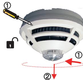
Push the locking peg in ① and turn device anticlockwise until it stops and then remove it from base ②.
