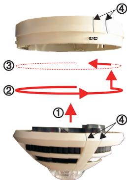
Offer device ① to base and rotate clockwise until it moves upwards on to the base ② and rotate again until it clicks and goes no further ③, the lines ④ on the base and device will align.
