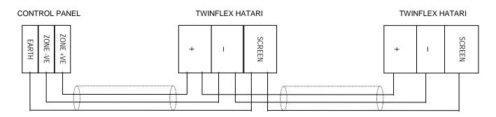
The Twinflex Hatari Sounder can be mixed on the same zone as other types of Twinflex device (eg. Twinflex Multipoint Detectors). The above diagram shows how to make the zone positive, zone negative and screen connections between the control panel and Twinflex Hatari Sounders. Refer to the instruction leaflets supplied with other Twinflex devices for their equivalent wiring/terminal labelling details.
