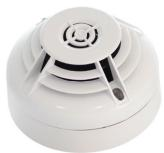
The sensing elements of the Opal NFXI-SMT2 are panel controllable so the sensitivity thresholds of each element can be changed by the panel offering the ability to customise the device for the changing use of the area it is protecting. The detector has built in short circuit isolation and two integral tri-colour LEDs that provide 360° local visual indication of the device status. The LEDs are programmable with static or blinking red, amber and green status indications available.
