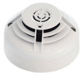
The sensing elements of the SMART<sup>3</sup> are panel controllable so the sensitivity thresholds of each element can be changed by the panel offering the ability to customise the device for the changing use of the area it is protecting. The detector has built in short circuit isolation and two integral tri-colour LEDs that provide 360° local visual indication of the device status. The LEDs are programmable with static or blinking red, amber and green status indications available.
